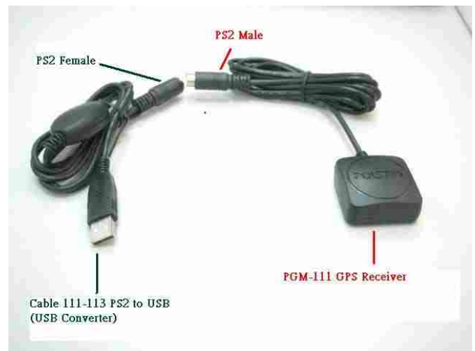
PGM-111 GPS with optional USB adapter cable. The cable includes an integrated USB to TTL converter.
